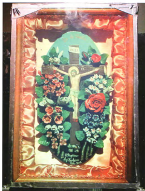
FIGURE 14.13 Full-colour Denisyuk reflection hologram made using the Z3 prototype portable RGB holography camera produced by the Hellenic Institute of Holography.
