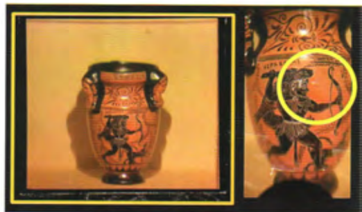
FIGURE 14.15 Full-colour Denisyuk reflection hologram of a Greek ceramic vase made by Yves Gentet. This analogue hologram was made in collaboration with the Hellenic Institute of Holography. The right-hand photograph shows an enlarged detail.
