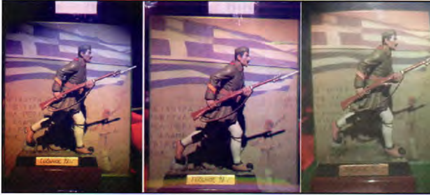
The same colour reflection hologram illuminated (L-R) with Holofos III, Holofos IV and tungsten halogen spotlights.
